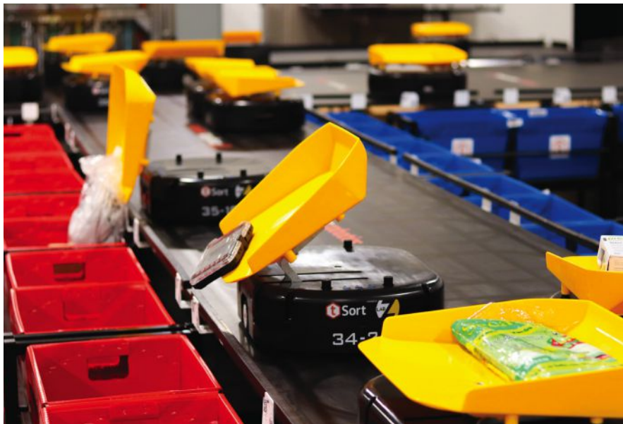
Mobile robotic solutions, like the one pictured here, allow grocers and retailers to sort orders that are batch picked in the store or a back room.
