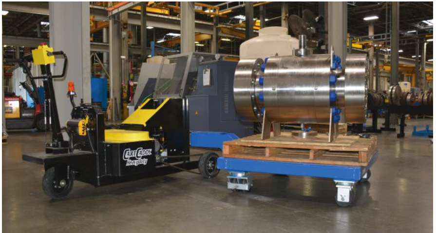
A 2500 class stainless steel valve on a transport cart. The cart is pushed using the heavy-duty Cart Daddy so operators can easily transport the valve to each operation.
