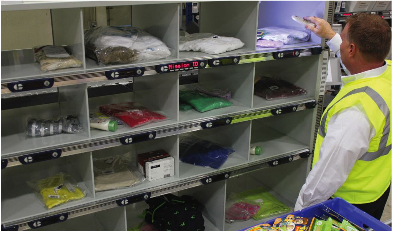
To support e-commerce and omni-channel fulfillment, the same put wall can support order assembly as well as returns.
