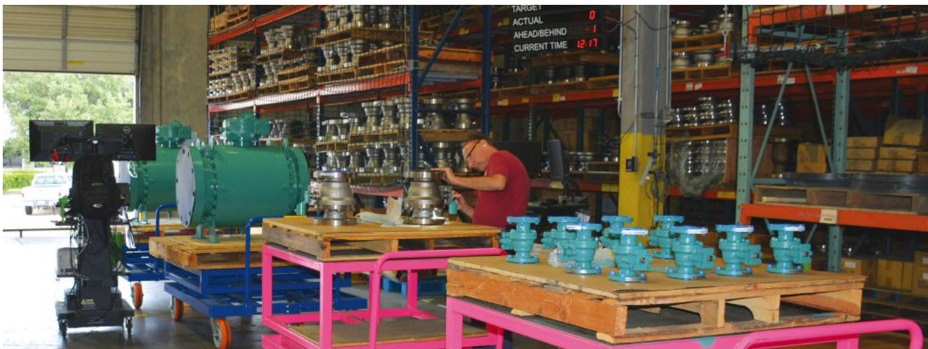
Frank Garcia, the flow master, inspects a job of valves before shipping. The finals process has two different types of carts for the various sizes of valves that flow through the area.
